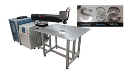
Questt Laser welding machine - Professional solution to the manufacture of Channel letter to make sidewalls and face or sidewalls and backwalls together.
